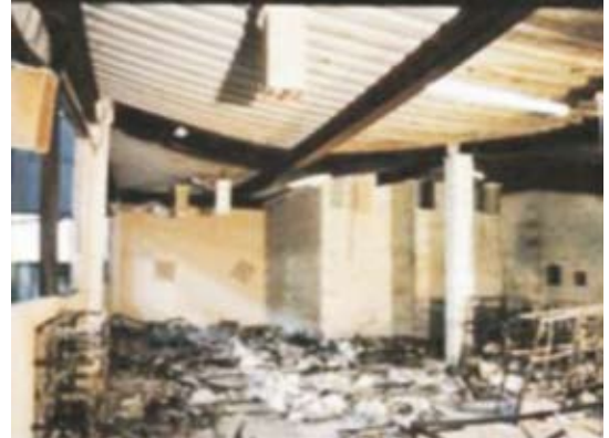
Resim 6.4. Cardinton, İngiltere yangın testi (Newman 2000) Corus Research Development & Technology
